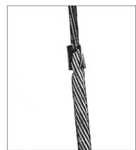
Drive the sleeve downward until the rods of the short leg are completely covered. The rods of the long leg should be even with, or may extend above the top edge of the sleeve.
